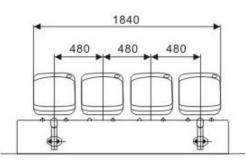
Chair faceplate: HDPE Connecting tube: galvanized tube Installation: wall mounted
