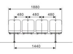
Chair faceplate: HDPE Connecting tube: galvanized tube Installation: floor mounted
