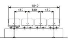
Chair faceplate: HDPE Connecting tube: galvanized tube Installation: floor mounted
